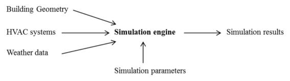
Figure 3 Input/output data of thermal simulation engine
