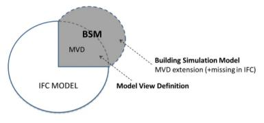
Figure 6 Building Simulation Model
