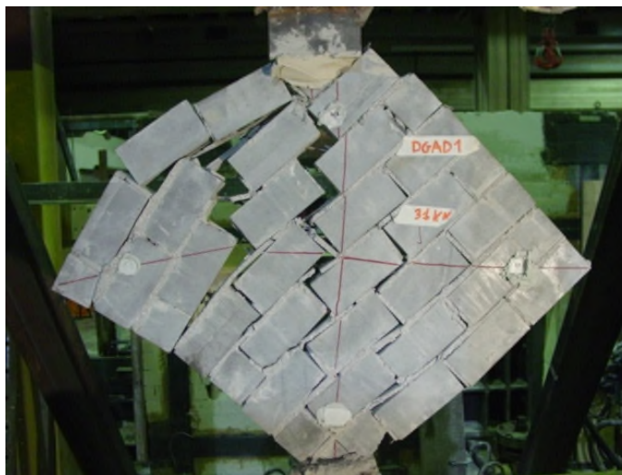
Figure 2 Reinforced panel, tested in diagonal compression, after breakage
