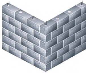
Figure 1 Reinforced masonry in natural stone
