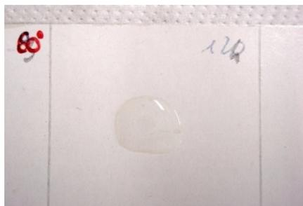
Figure 1 Oil drop on treated paperboard with CIPACK's coating
