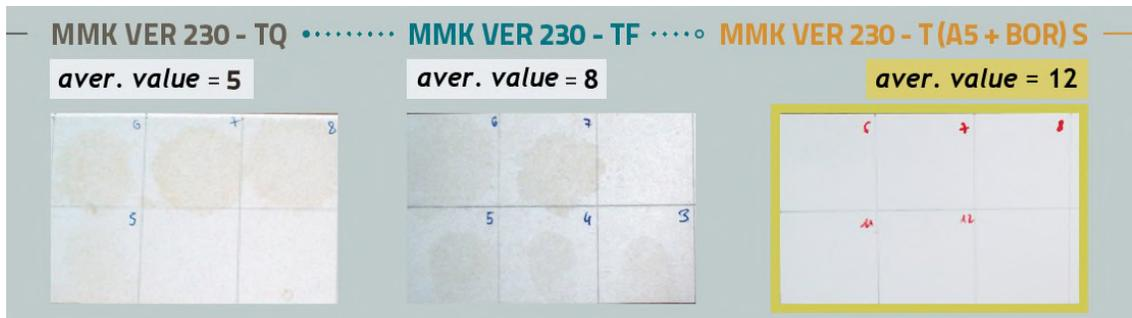
Figure 7 Comparison between the level of oil absorption (Kit Test - TAPPI 559) of uncoated paperboard (sx), fluorinated paperboard (c) and natural-based coatings (dx) on virgin fibre based materials
