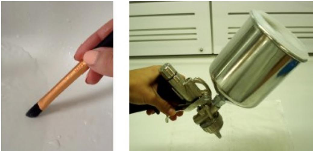
Figure 6 Brushing and spray coating deposition
