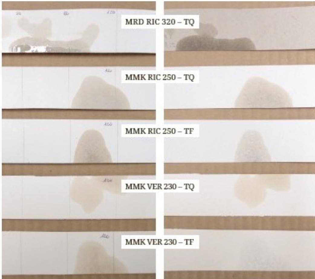
Figure 9 Level of oil absorption in critical temperature conditions ( $120^{\circ}\text{C}$ ) after 120 minutes. Comparison between uncoated (TQ) and fluorinated paperboard (TF)
