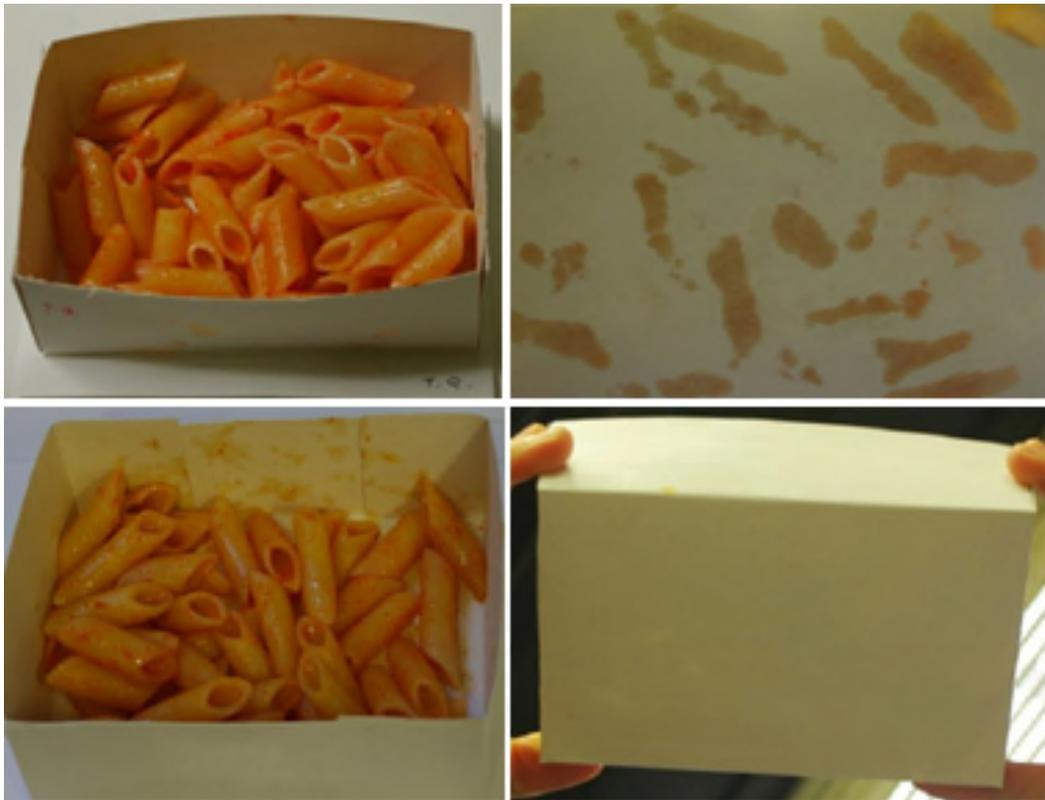
Figure 2 Non-coated paperboard (up) and oil-repellent CIPACK's coated paperboard (down)
