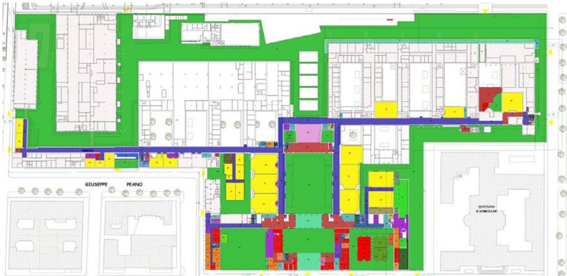
Figure 8 The Main campus (administrative offices) test of uploading data from the preliminary model built with Revit Architecture to the 2D CAD drawings supported in Archibus (by Daniele Dalmasso)
